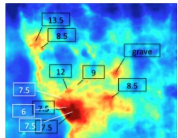
Measuring the defects (in mm) via the pin test (below) by experts of Opificio.
